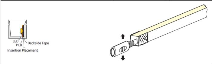
4. Insert the connector pins into the gap created by the inducer on the backside of the PCB, and push in.
